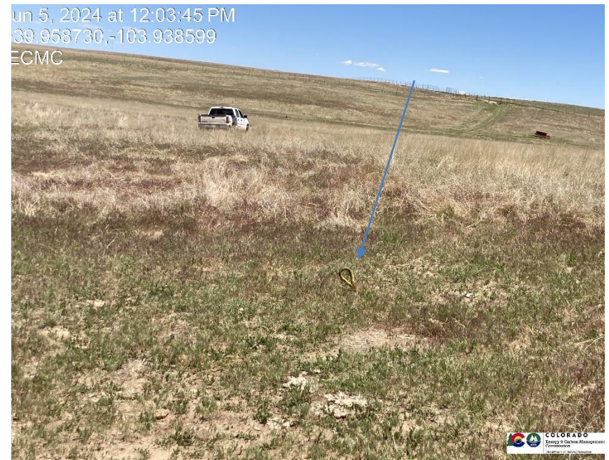
Pic 6 Deadman anchor is not marked
