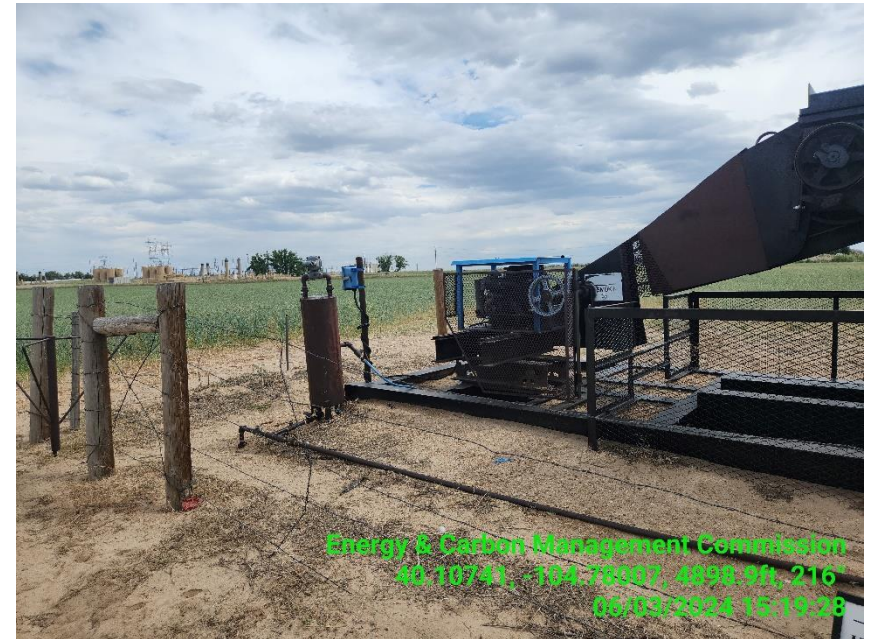
Photo 4 Prime mover/gas engine.
