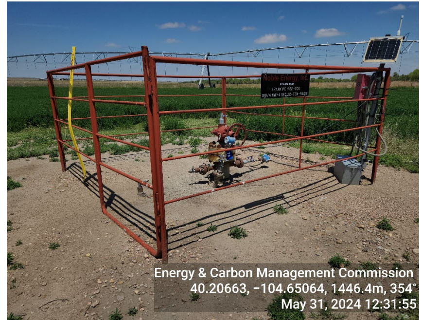
Photo 6: TA wellhead
