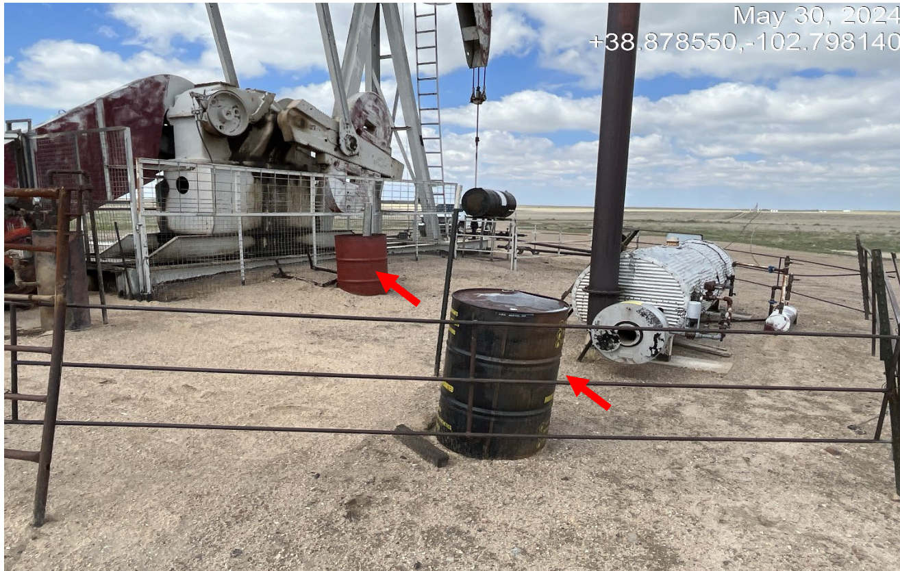
Photo 6. There are chemical barrels with no secondary containment. There is fresh sand spread around the pumjack where oil staining was previously observed.
