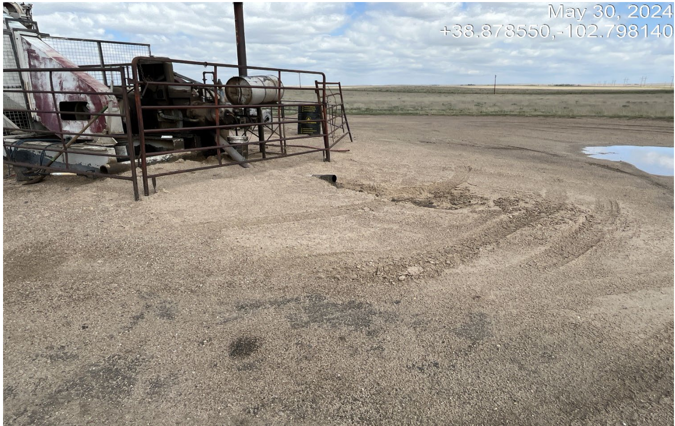
Photo 7. Facing at the backside of the pumpjack where exhaust is located. There is fresh sand spread around the exhaust pipe where oil staining was previously observed.
