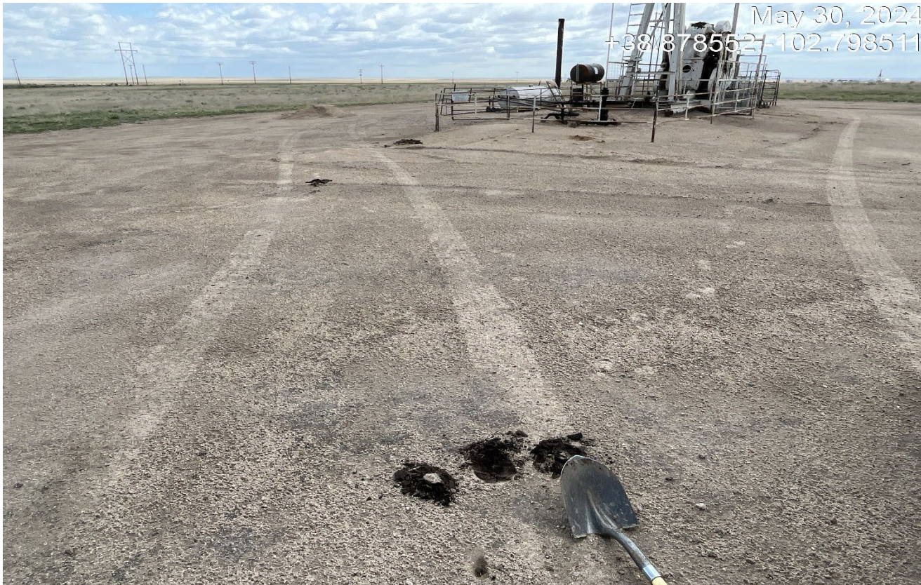
Photo 5. Further out from the well just a few inches below the surface was oil stained soils with a hydro carbon odor. All impacted soils must be cleaned up and removed.
