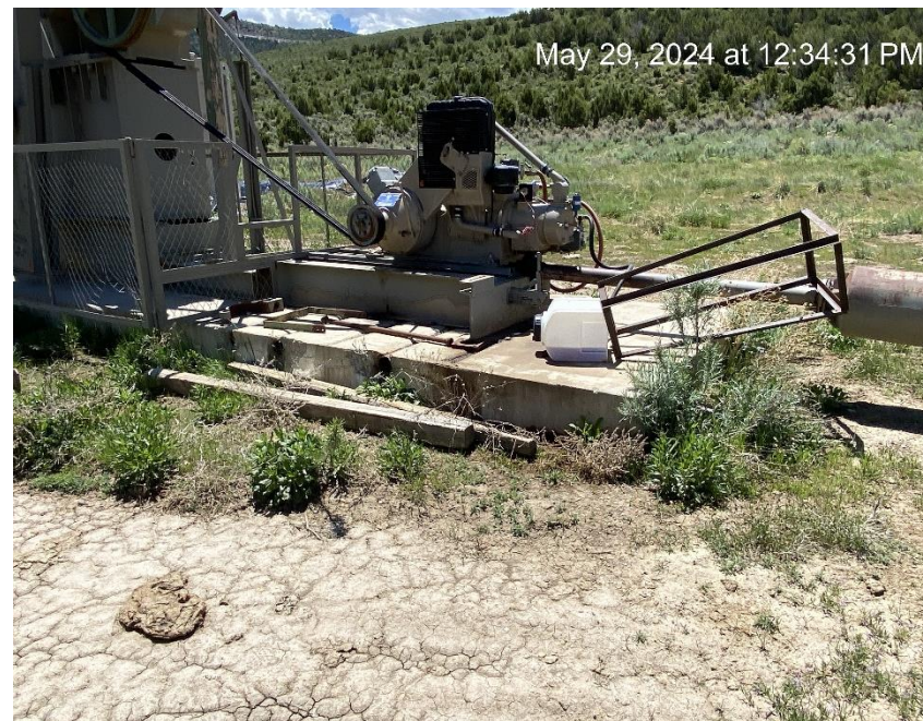
Debris. No containment. Leaking container.
