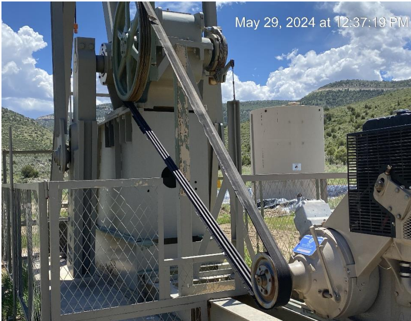
Belt guard missing creating human and wildlife hazard
