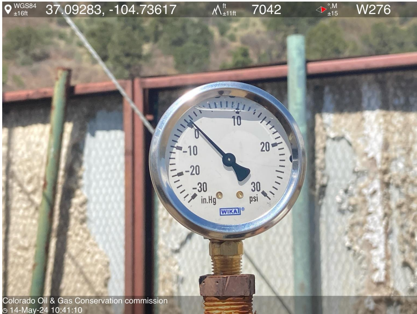
PHOTO 5: INJECTION PRESSURE 0 PSI, WELL WAS NOT INJECTING AT TIME OF INSPECTION.
