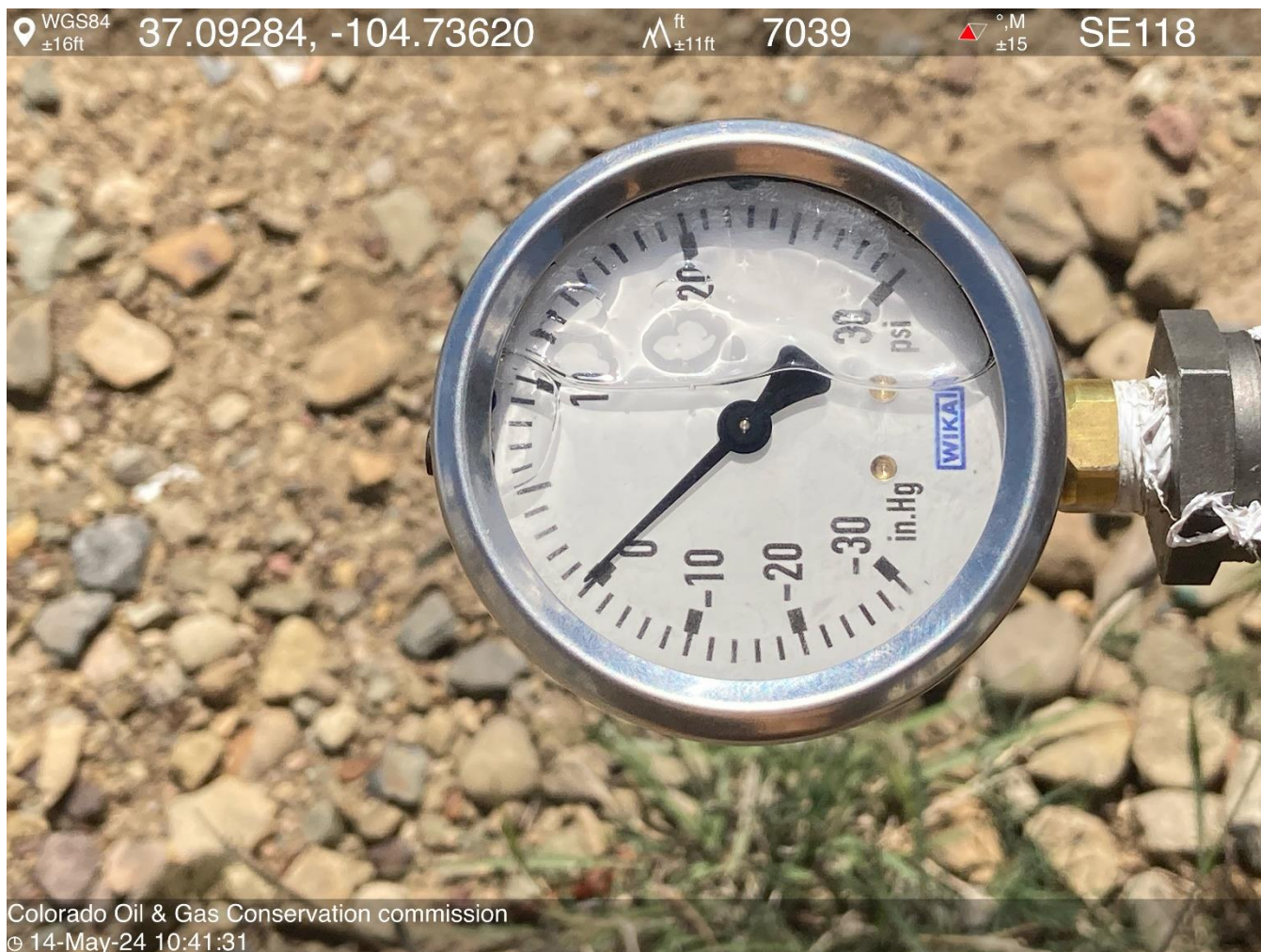
PHOTO 7: BRADENHEAD 0 PSI, BLEW DOWN IN 5 SECONDS NO BLOW NO FLOW.
