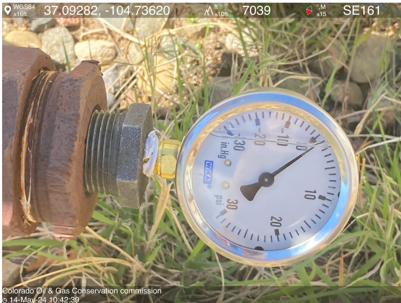
PHOTO 6: TBG/CSG 2 PSI, BLEW DOWN IN 5 SECONDS NO BLOW NO FLOW.
