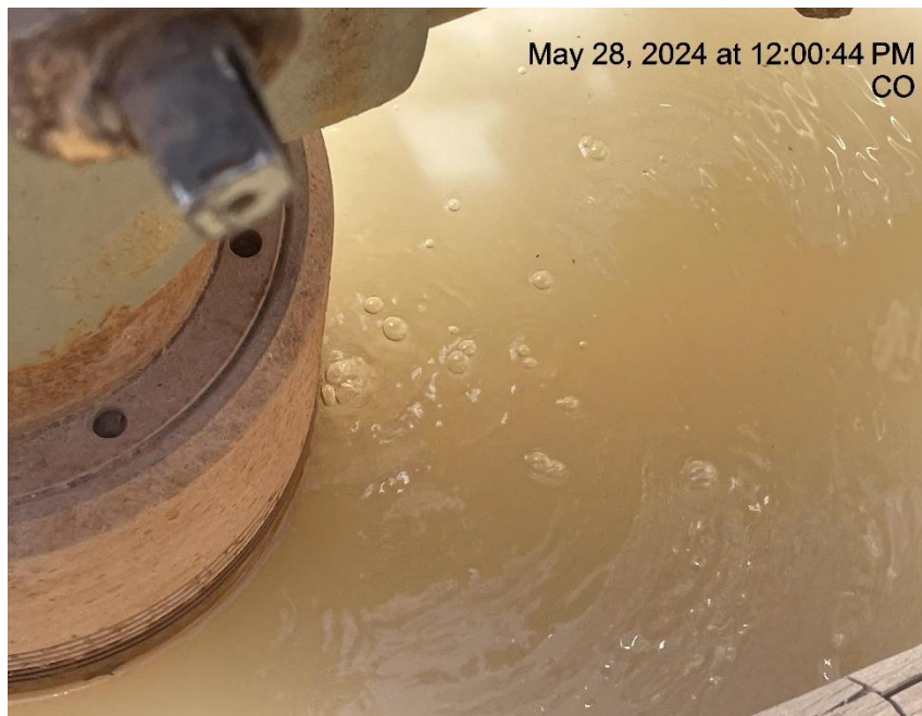
Photo # 8447 Possible wellhead leak/gas bubbling up around wellhead through water in cellar
