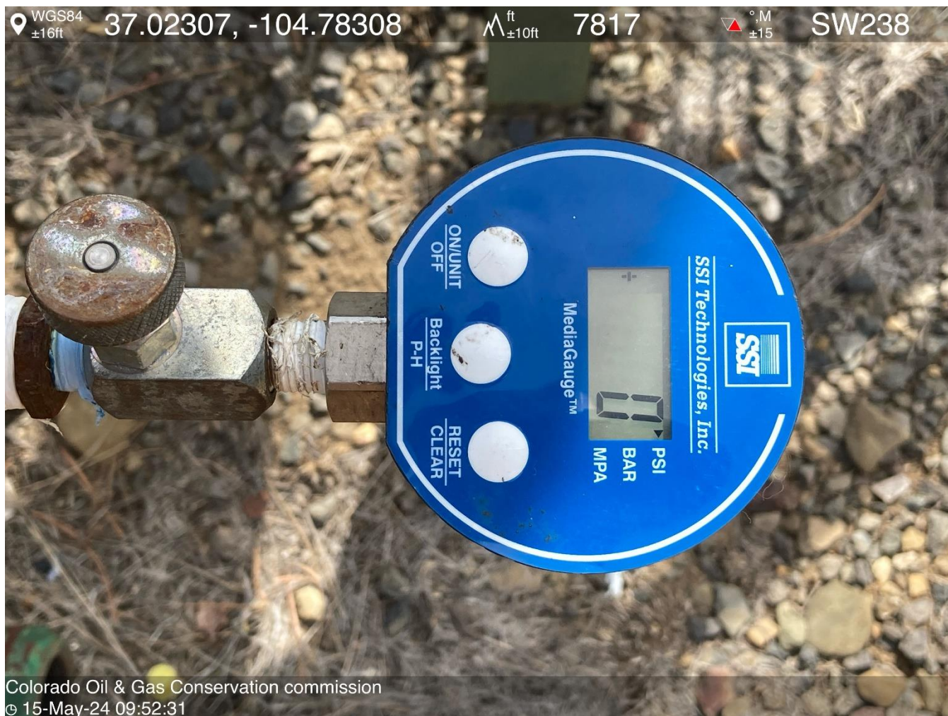
PHOTO 4: TBG/CSG ANNULUS 0 PSI
