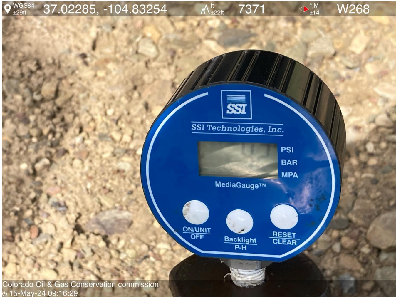
PHOTO 5: BRADENHEAD HAD 42 PSI, BLEW DOWN IN APP. 60 SECONDS MONNITORED FOR 15 MIN. BO BLOW NO FLOW.
