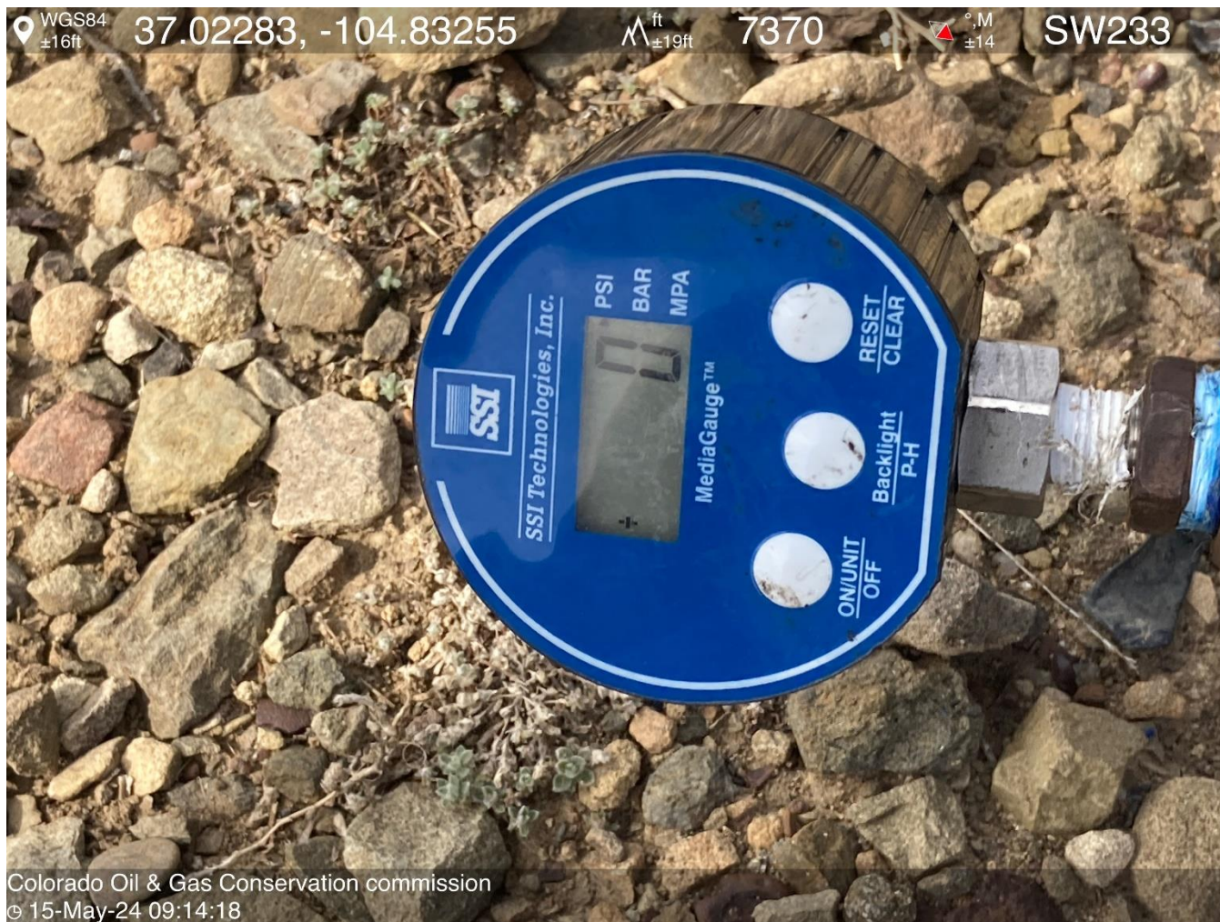
PHOTO 4: TBG/CSG ANNULUS 0 PSI.
