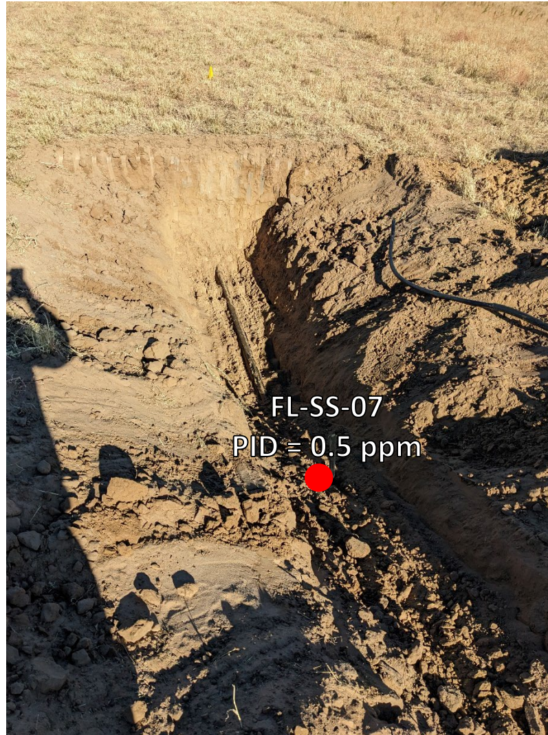
Looking northwest at bellhole/cutpoint No petroleum hydrocarbon staining or odor observed
