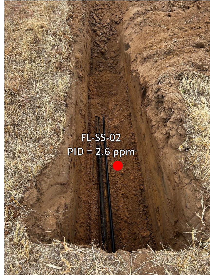
Looking northwest at bellhole/cutpoint No petroleum hydrocarbon staining or odor observed
