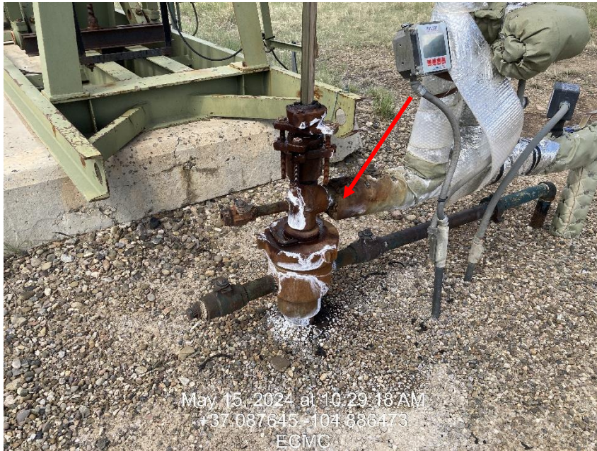
Photo 7 – Stains on Wellhead
