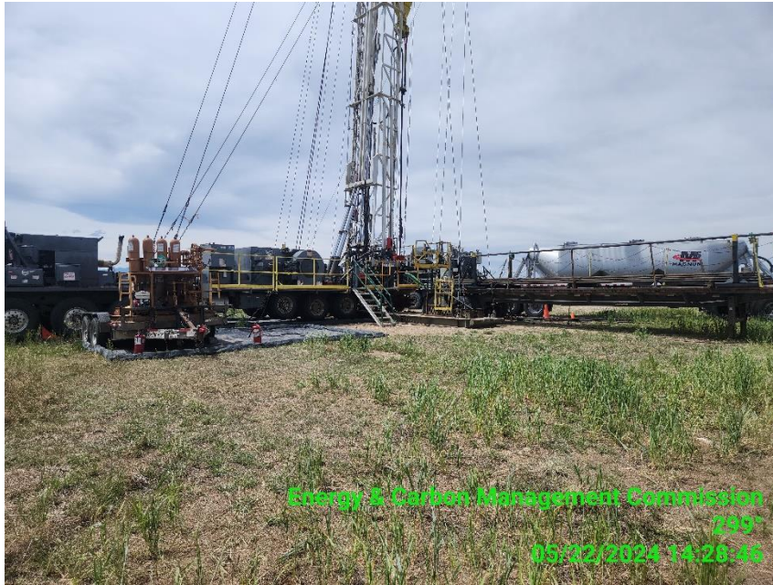
Photo 5 WO Rig, accumulator trailer & pipe trailer.
