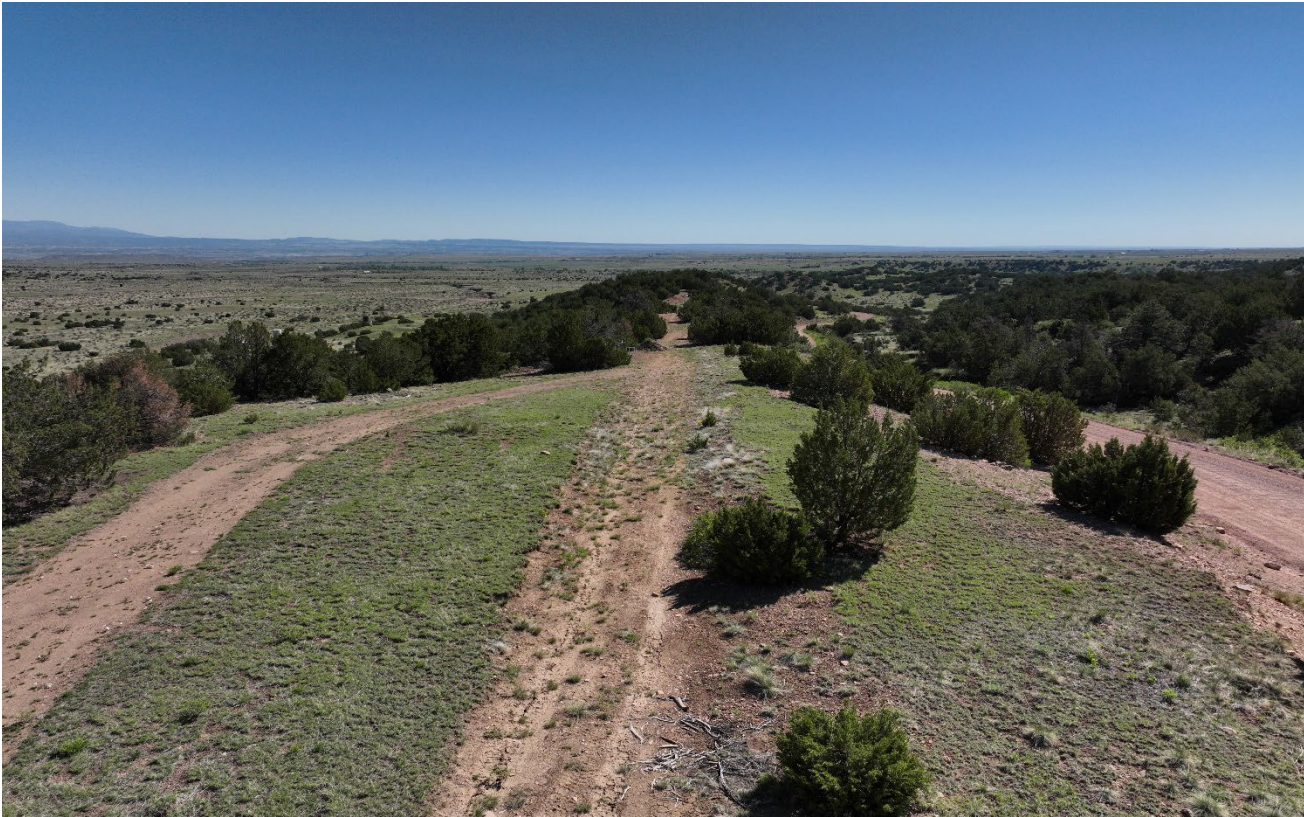
Photo 1. Drone aerial photo facing northeast. There is a new road built on the left side however the original access road remain unreclaimed in center of the photo.
