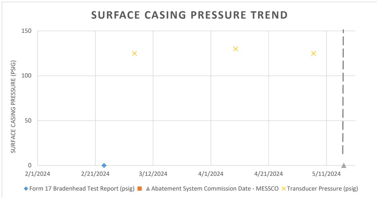
**Comments:** February 2024 initial rig release test had 0 PSI with no flow or pressure for entire test. However, monthly monitoring data has been above threshold. Based on monthly monitoring data, PDC has installed a MESSCO abatement system to remediate bradenhead pressure. A sample was collected 5/20/2024 and a new form 17 test has been requested following a 7 day abatement shut-in. PDC will continue to remediate pressure using the installed abatement system and reevaluate in 6 months.
