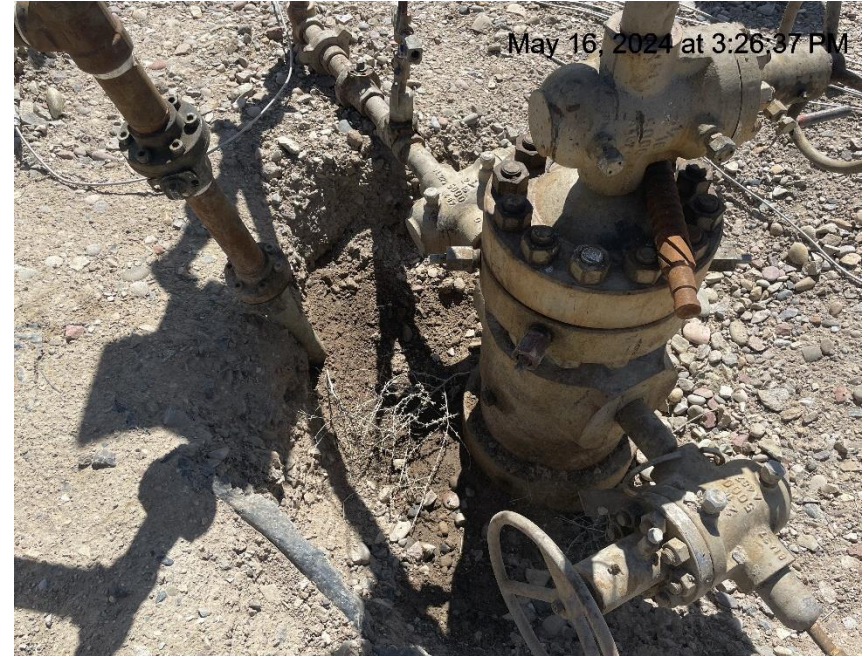
Photo # 7560 Staining around wellhead
