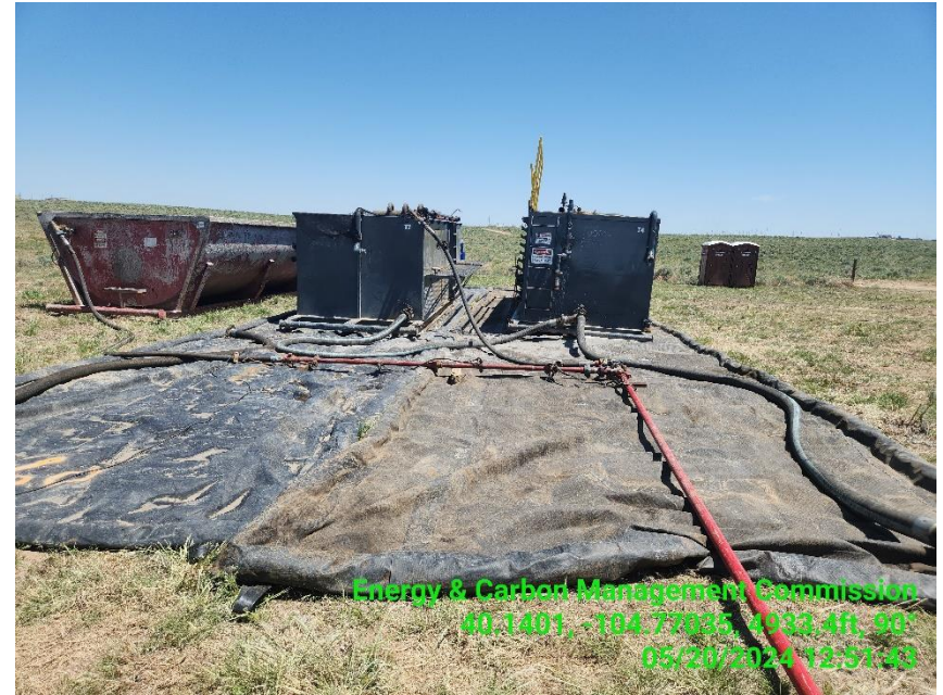
Photo 4 Circulation tanks.
