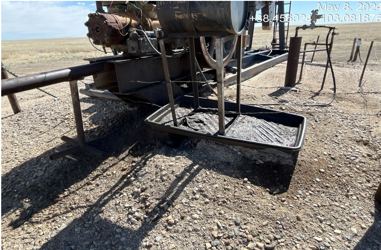
Photo 5. There is oily fluid in the containment next to the pump jack. Oily fluid has spilled onto the ground and needs to be cleaned up. Previous corrective action was not completed. Netting must be installed to prevent wildlife entry.
