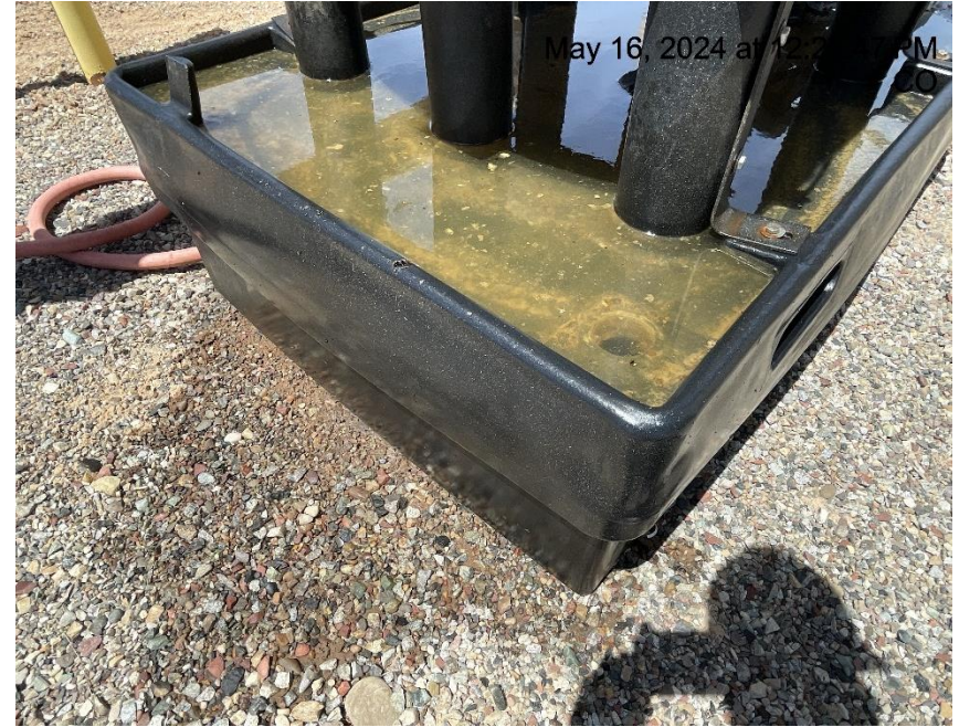
Photo # 7436 Failure to maintain chemical BMP - Chemical tank containment full of fluid/fluid overflowed containment & spilled on the ground
