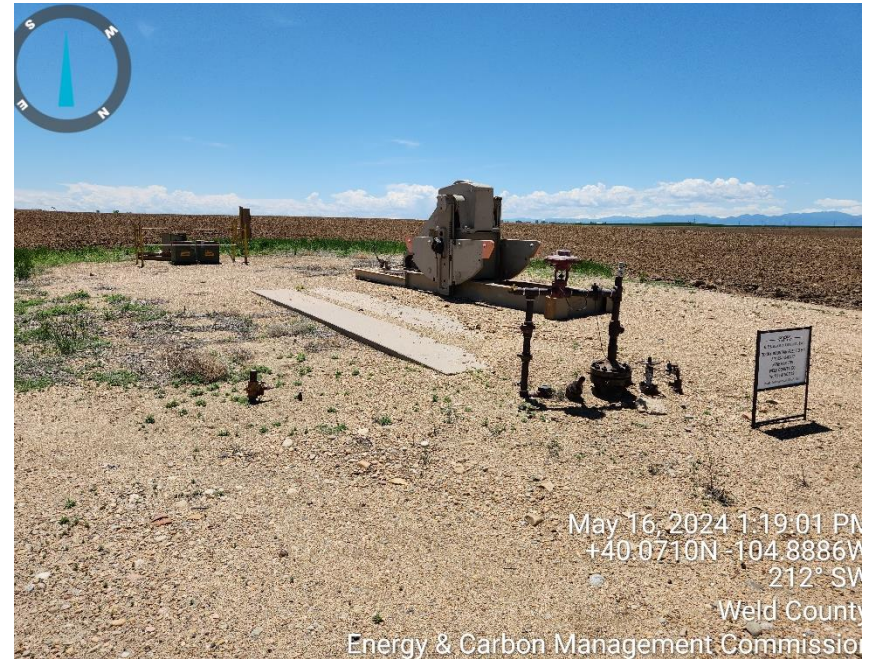
Photo 2 well head and equipment, disassembled pumping unit
