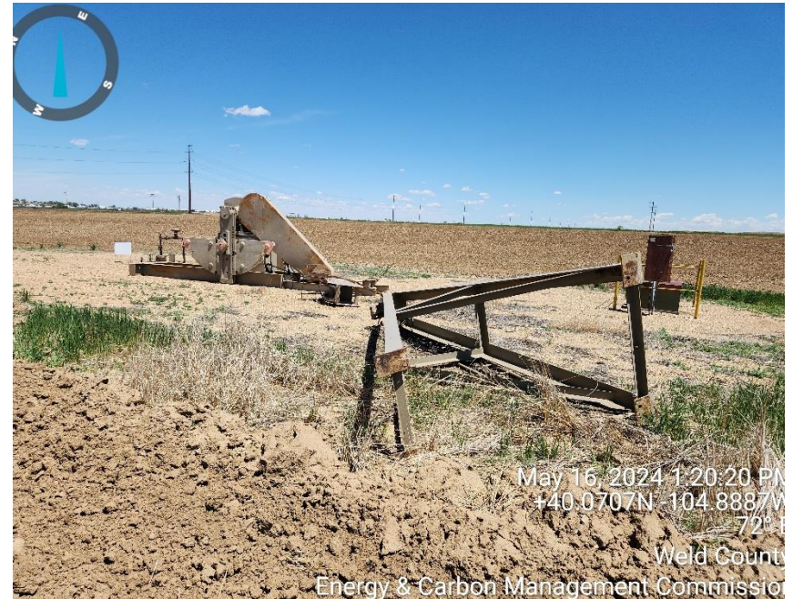
Photo 4 disassembled pumping unit
