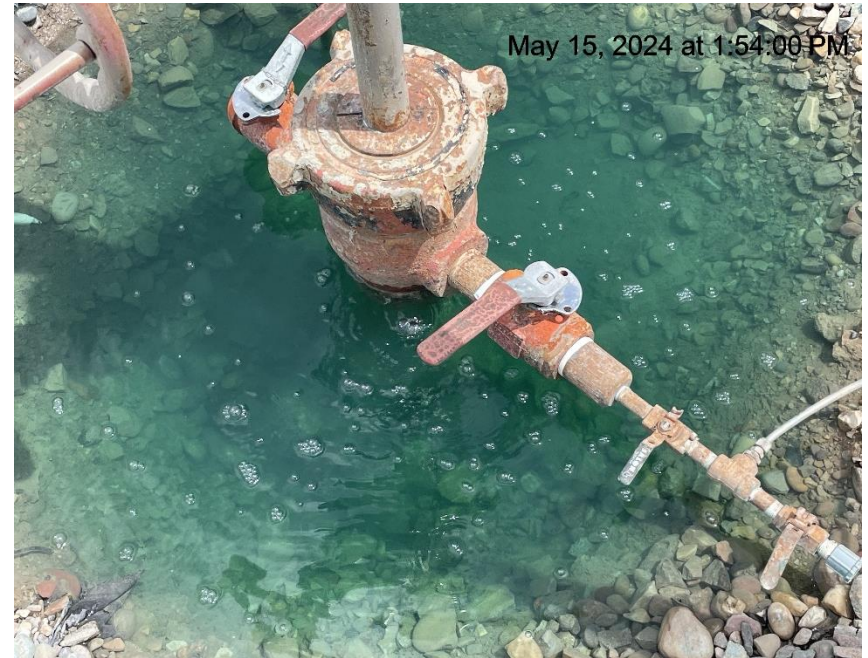
Photo # 7064 Possible wellhead leak on W 15-5 well
