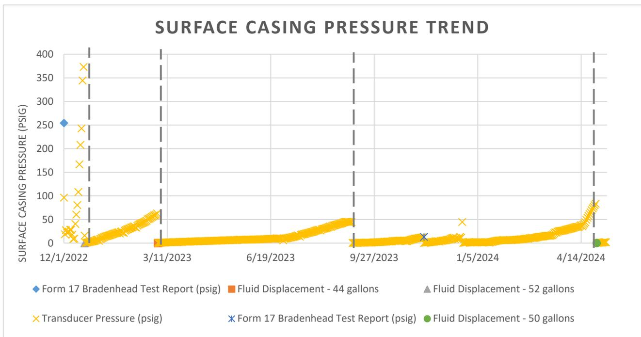
**Comments:** 2022 1st post-production test had 254 PSI that blew down to 0 psi after the first minute with no flow for the remainder of the test. November 2023 annual test had 13 PSI that blew down to 0 PSI in seconds with no flow or pressure for the entire test. Bradenhead gas determined to be thermogenic gas with somewhat similar composition as the production gas sample. PDC will continue to remediate pressure using fluid displacement.
