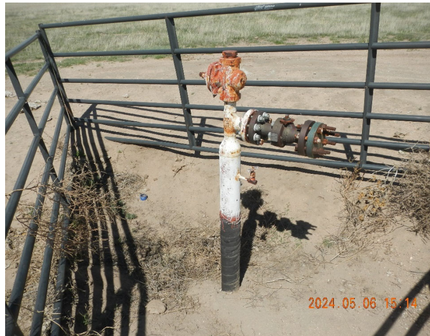
4. Flowline riser with valves and plugs.
