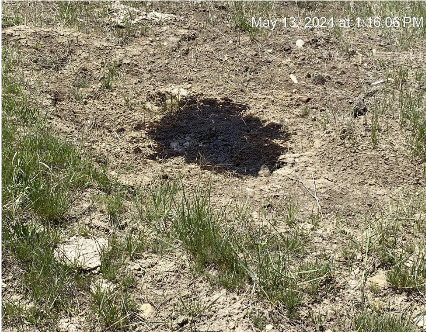
Oil seepage downhill from wellhead. Cellar leak?
