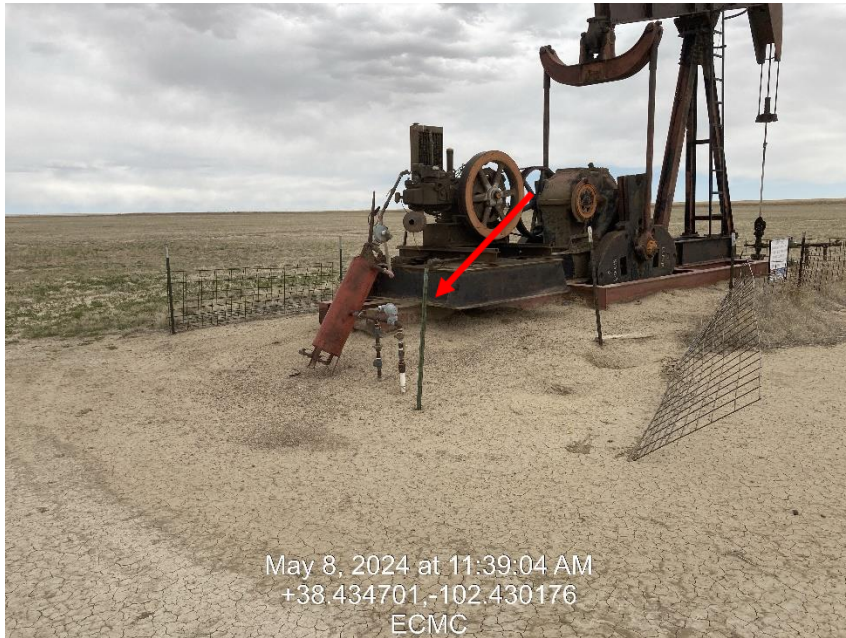
Photo 3 – Machine Guarding not maintained
