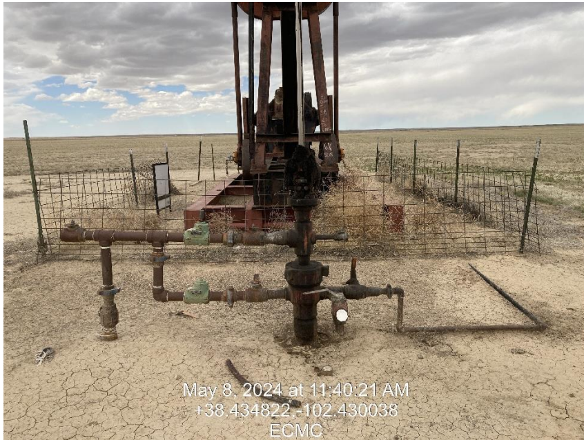
Photo 5 – Well head with rag on stuffing box
