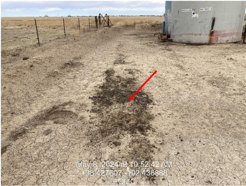
Photo 9 – Impacted soils in Secondary Containment
