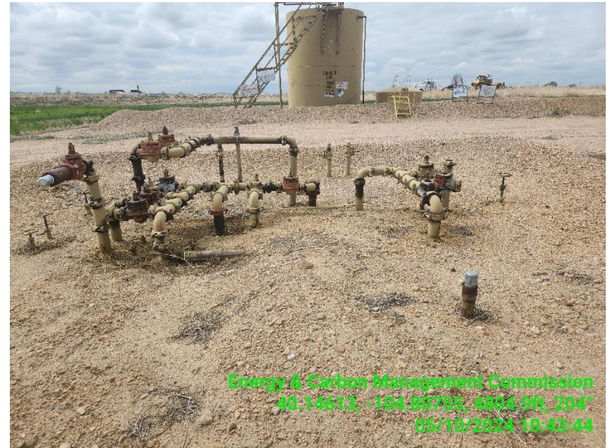
Photo 4 Flow line manifold.
