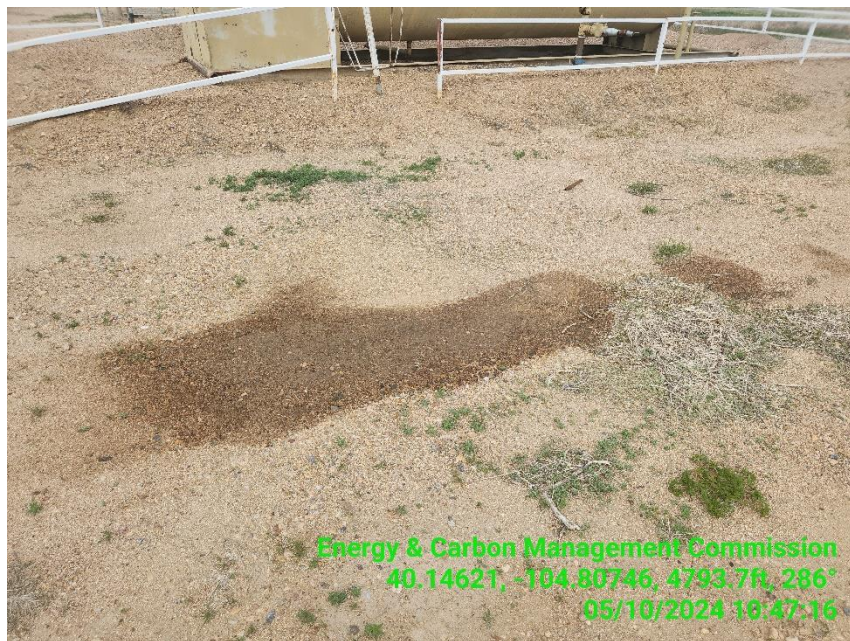
Photo 9 Stained soil to the west of the Horizontal Heater Treater.
