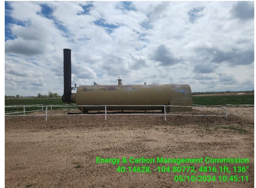
Photo 6 Horizontal heater treater.
