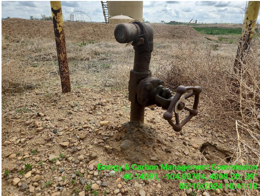
Photo 13 Stained soil around flow line riser west of the TB.
