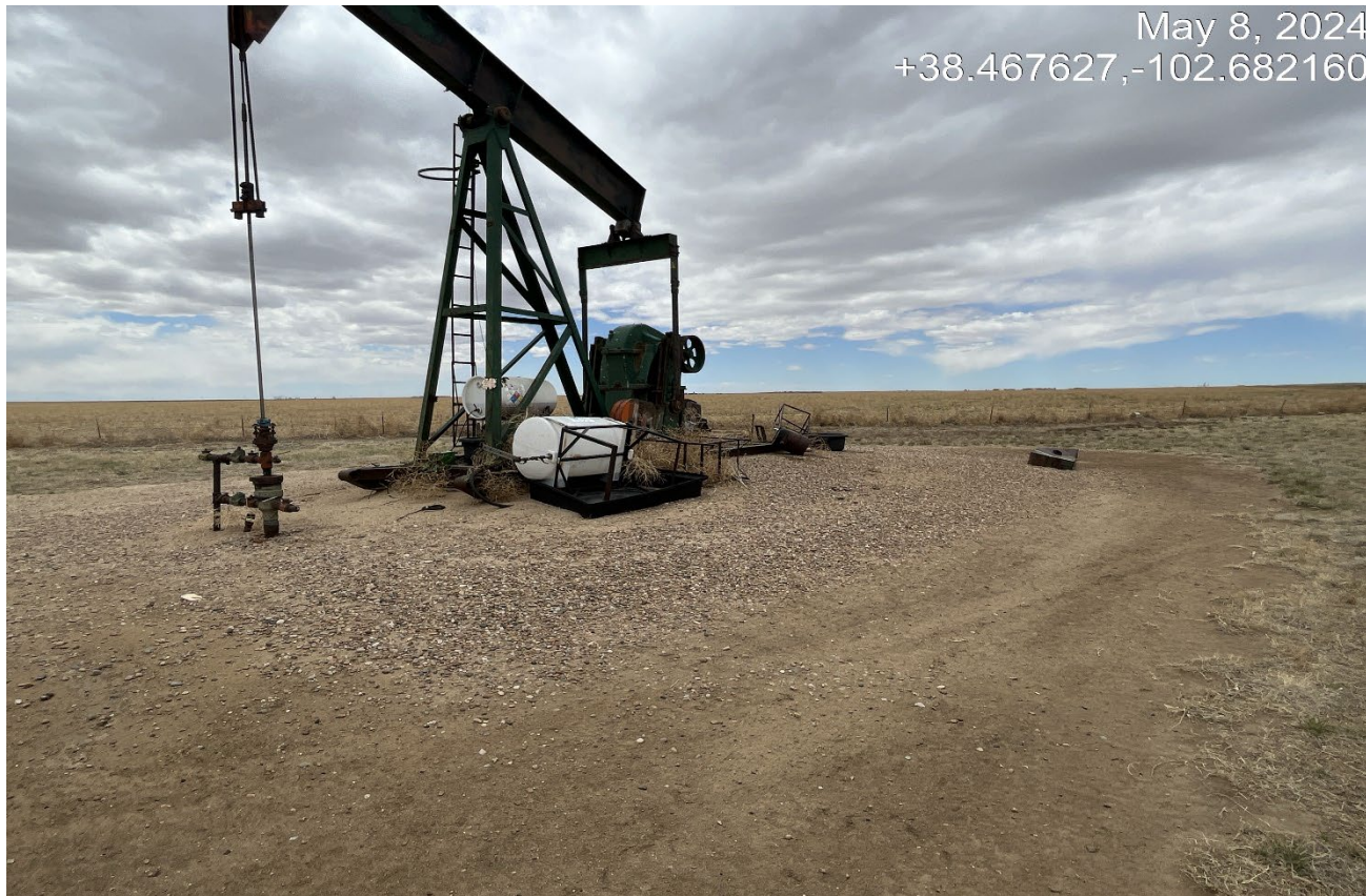
Photo 3. Facing toward the wellsite. The chemical container has tipped over.
