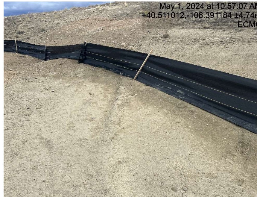
Silt fence failing
