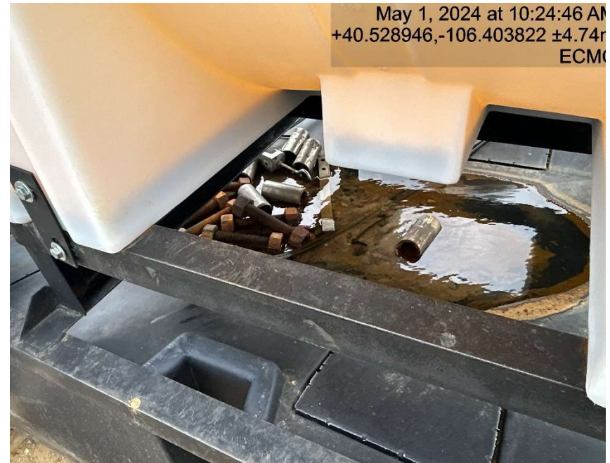
Debris and chemical containment full of fluid
