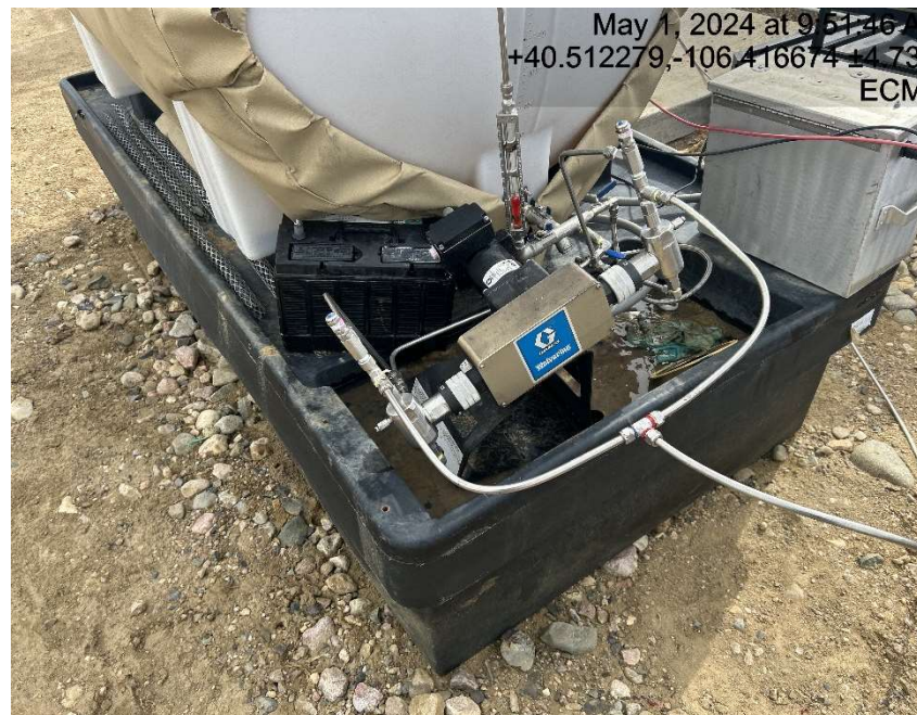
Debris and containment full of fluid
