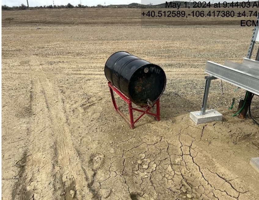
Unknown tank and not in secondary containment
