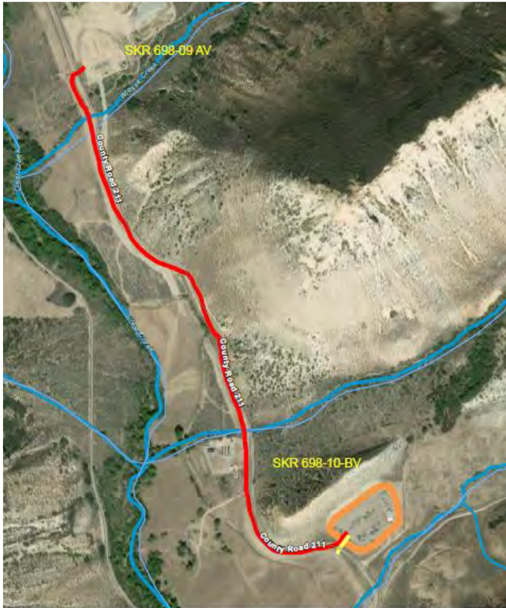
FIGURE 3- Liquids (Red) and Gas (Yellow) Flowline Tie-in; SKR 698-10-BV Well Pad to the SKR 698-09-AV Well Pad
