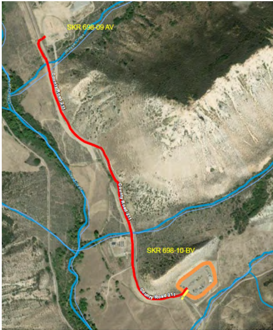
FIGURE 2- Liquids (Red) and Gas (Yellow) Flowline Tie-in; SKR 698-10-BV Well Pad to the SKR 698-09-AV Well Pad
