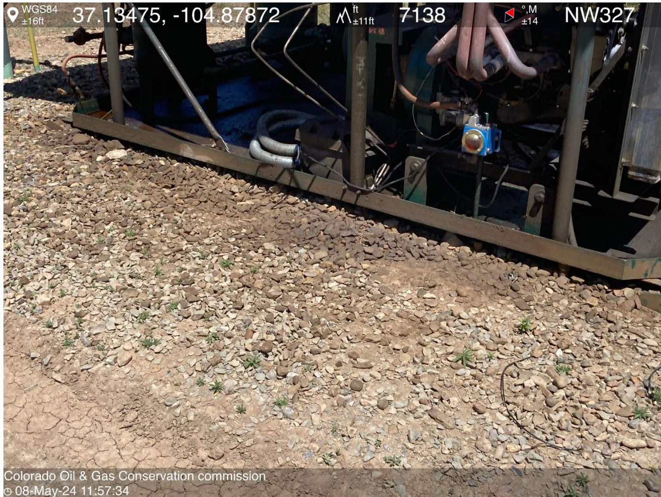
PHOTO 5: AREA OF IMPACTED SOIL NEAR COMPRESSOR SKID. Conduct maintenance on equipment, cleanup stained material and review self inspection processes. COMPLY WITH RULE 1002,.(2).D. CA DATE 6-8-2024.
