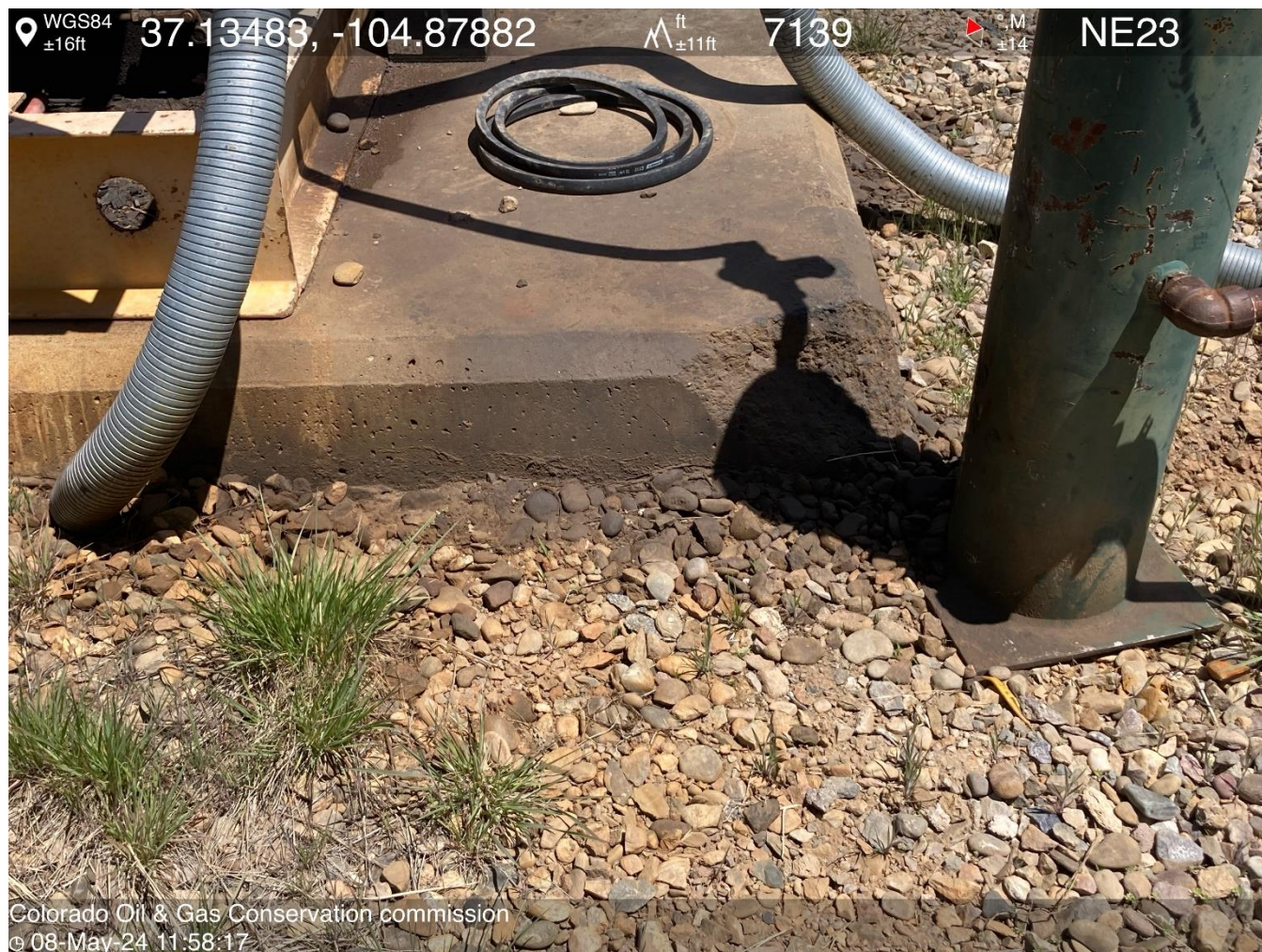
PHOTO 6: AREA OF IMPACTED SOIL NEAR PUMPJACK SKID. Conduct maintenance on equipment, cleanup stained material and review self inspection processes. COMPLY WITH RULE 1002,.(2).D. CA DATE 6-8-2024.
