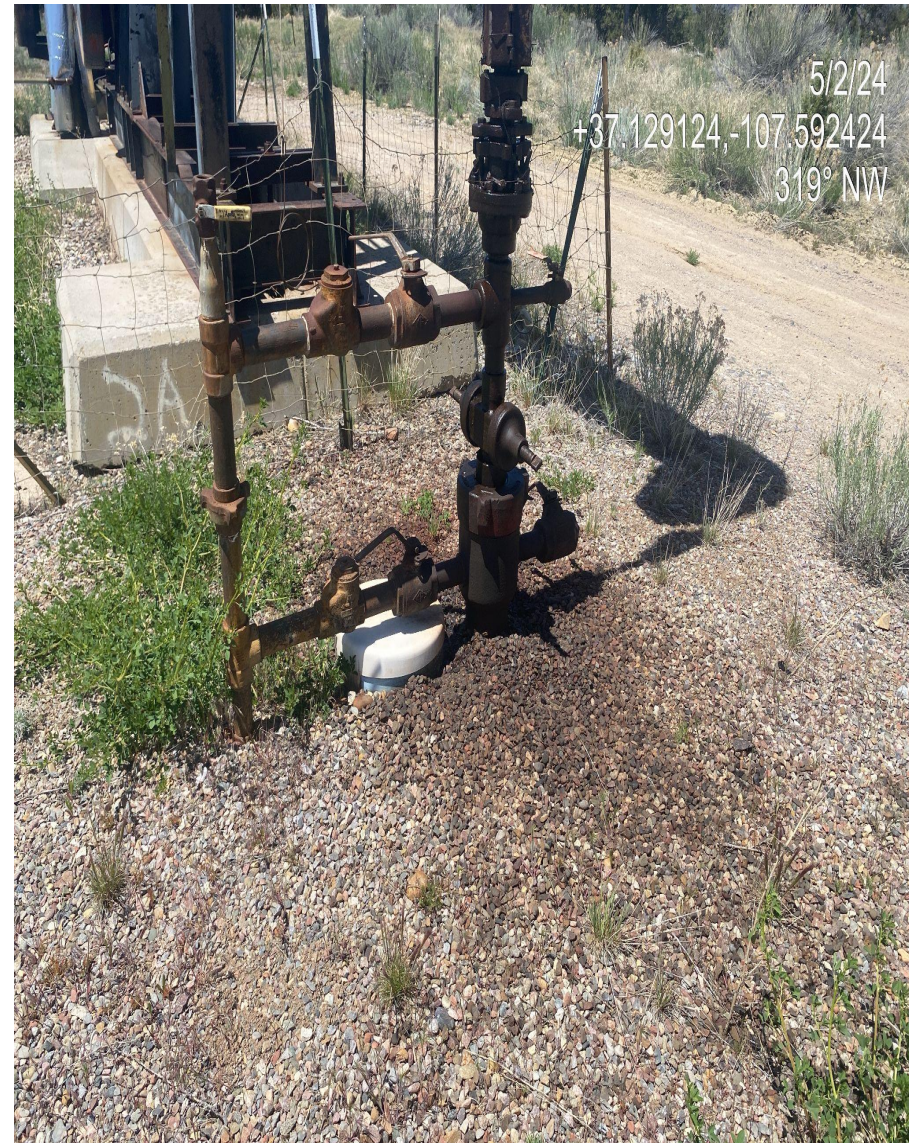
Photo 2. Impacted surface material remains at both well heads.
