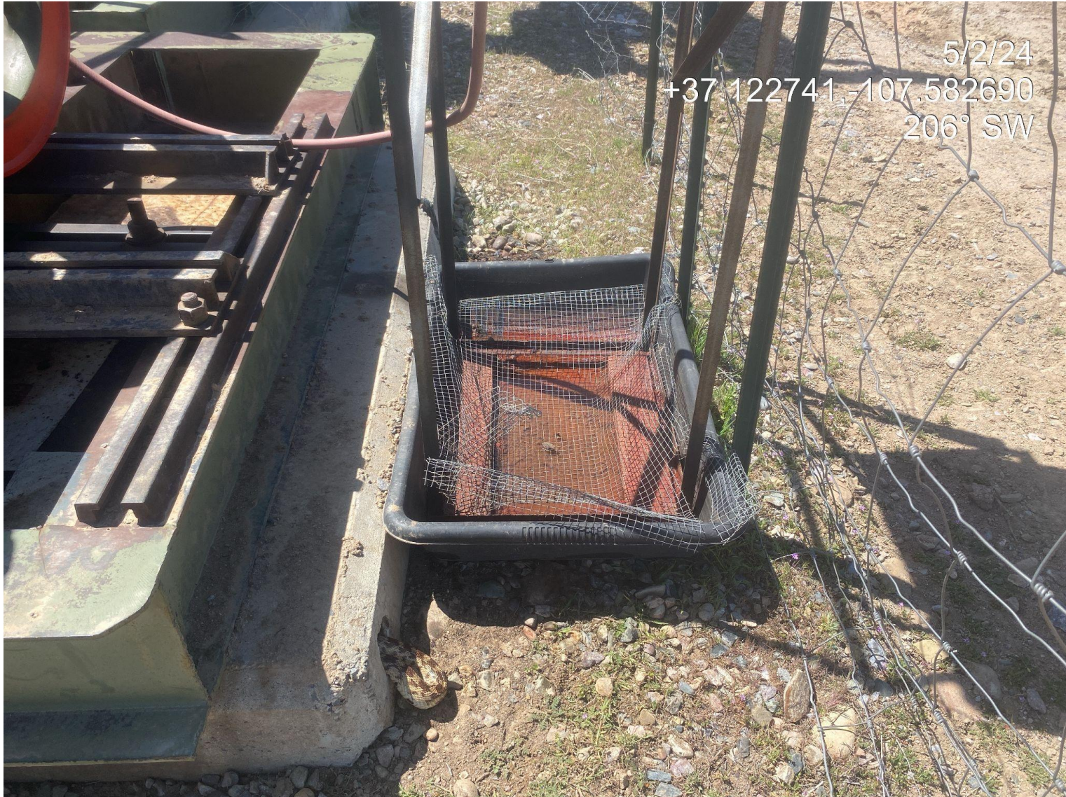
Photo 3. View of wildlife netting at lube oil tank secondary containment that is no longer functioning.
