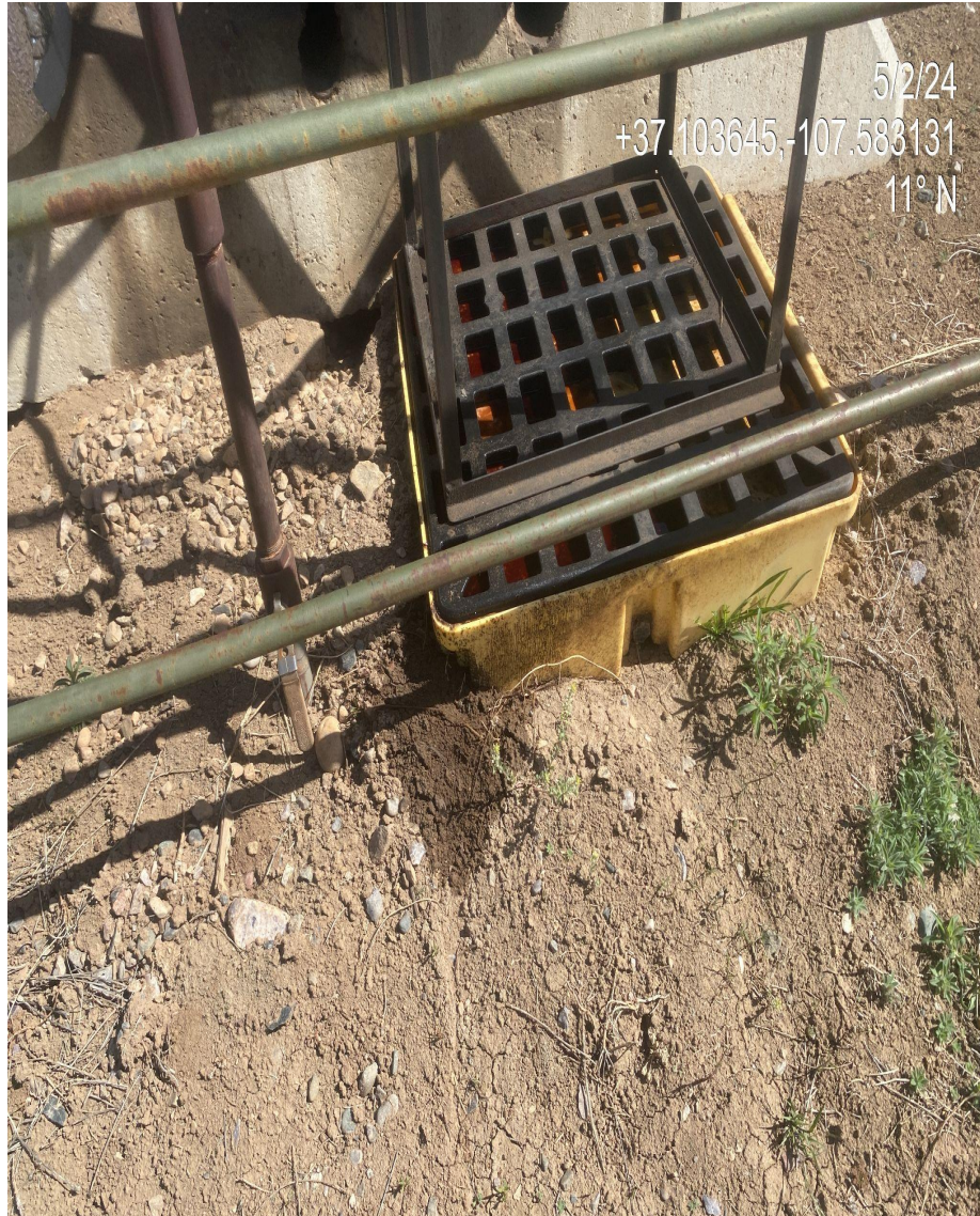
Photo 7. View of impacted surface material at both lube oil tanks secondary containments at both pump jacks.
