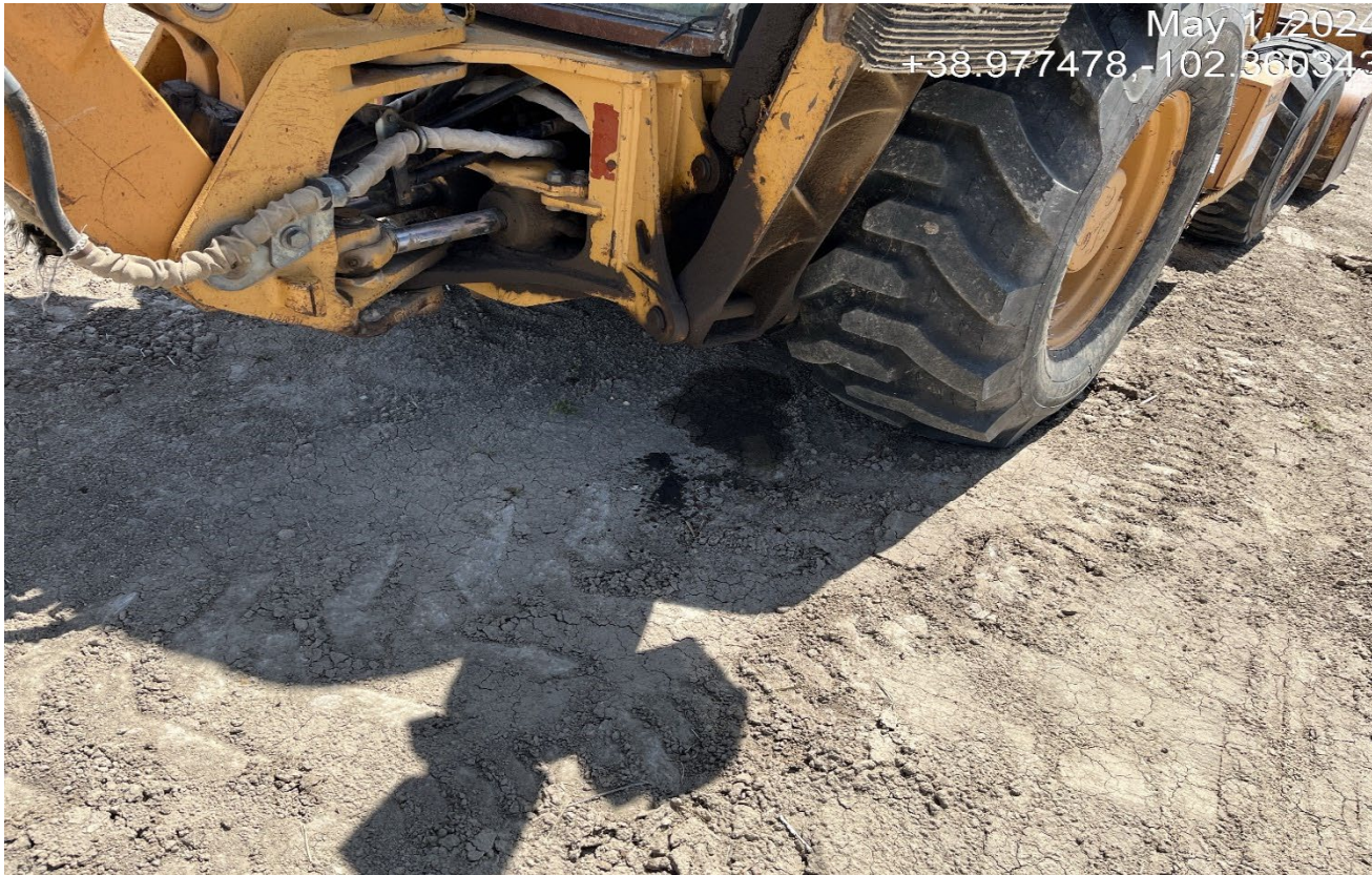
Photo 4. The backhoe onsite is leaking oil which needs to be cleaned up.
