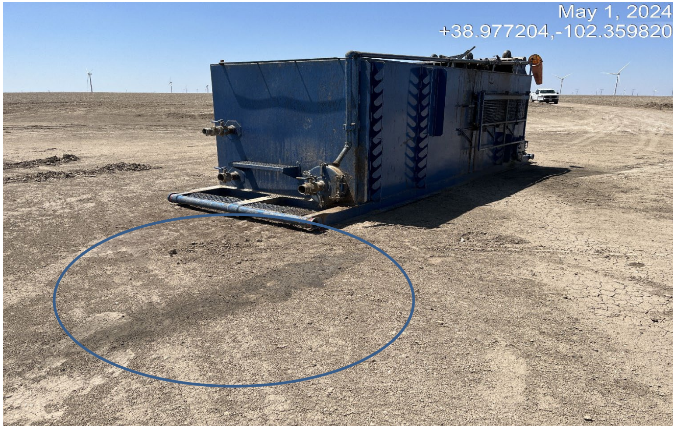
Photo 9. Facing toward the open top tank. There are stained soils shown in the circled area near the tank..
