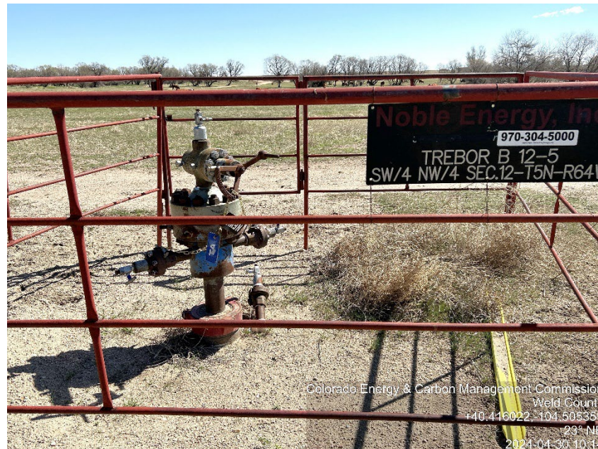
Photo #2 Trebor B12-5 (123-13776) Wellsite Temporarily Abandoned | TA
