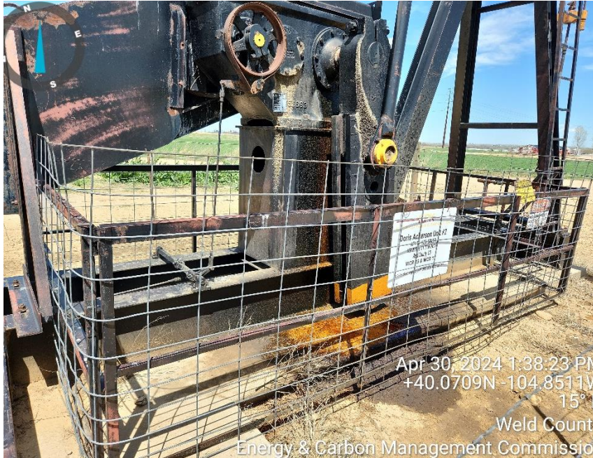
Photo 1 gear box leak on pumping unit
