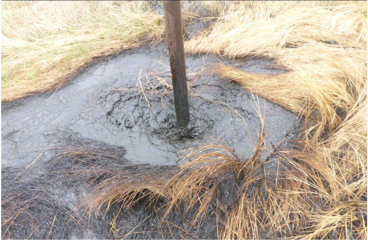
Base of the riser. Shows contraction indicating there is no longer a discharge.
