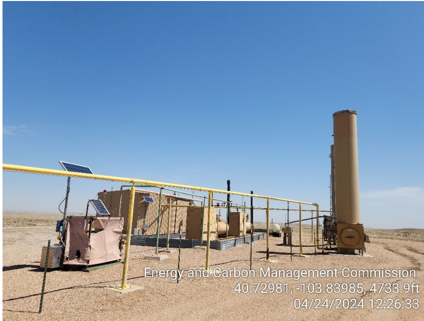
Photo 5 – VRU and Separators
