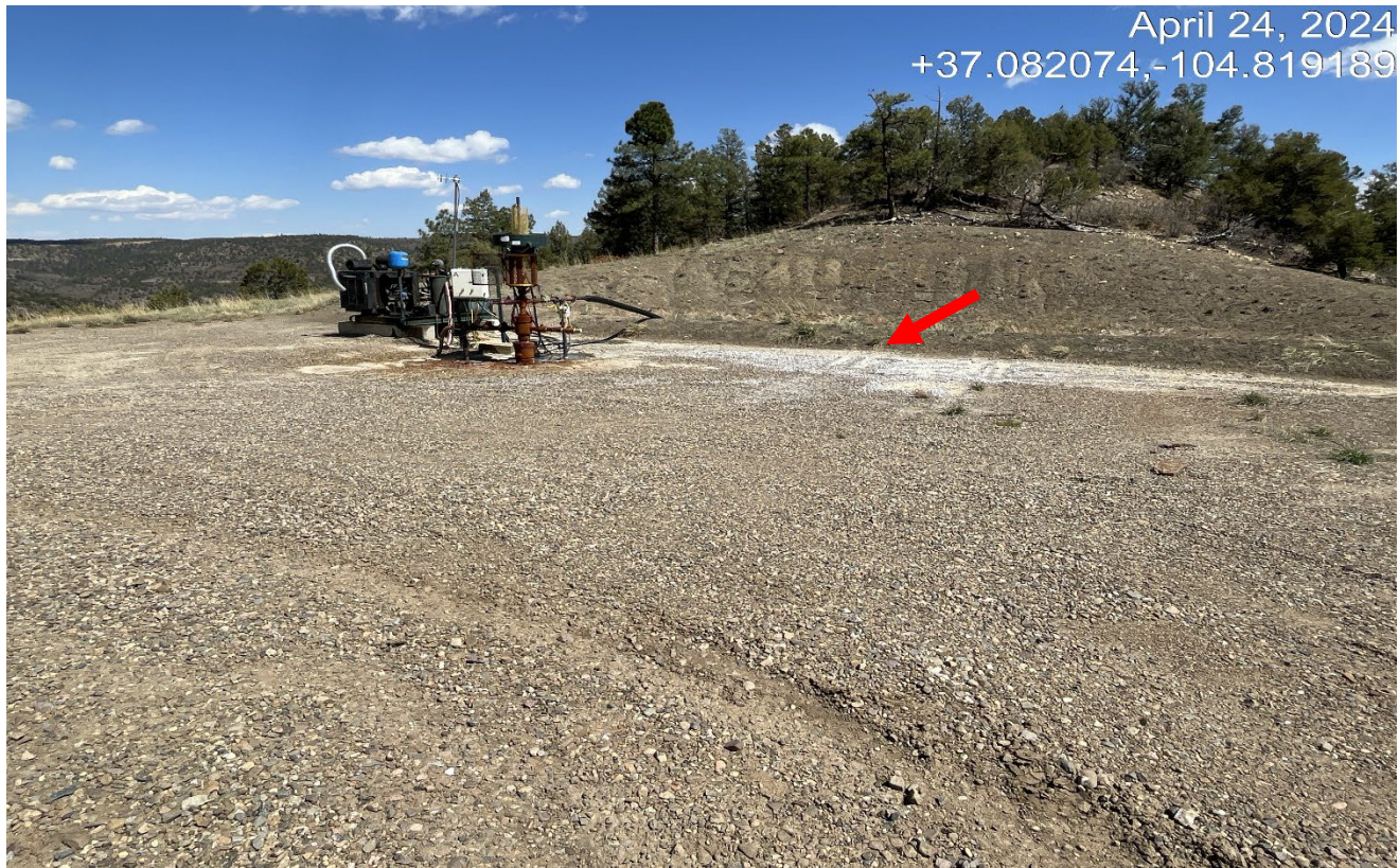
Photo 1. Facing northeast toward the wellsite. There was a leak at the wellhead that left a white residue.
