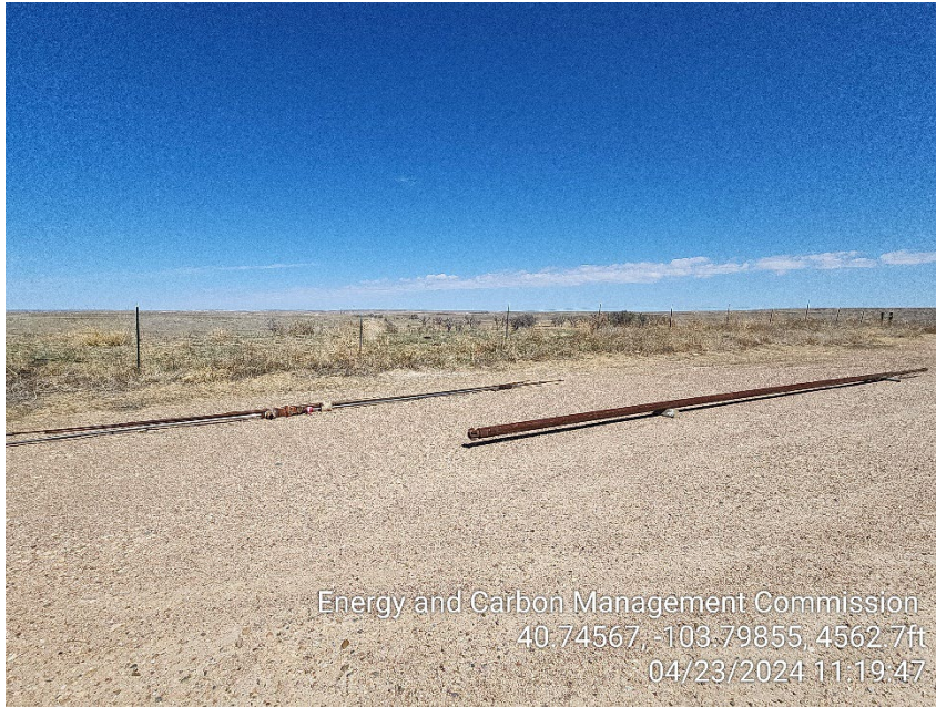
Photo 5 – Unused Down Hole Tools and Polish Rod
