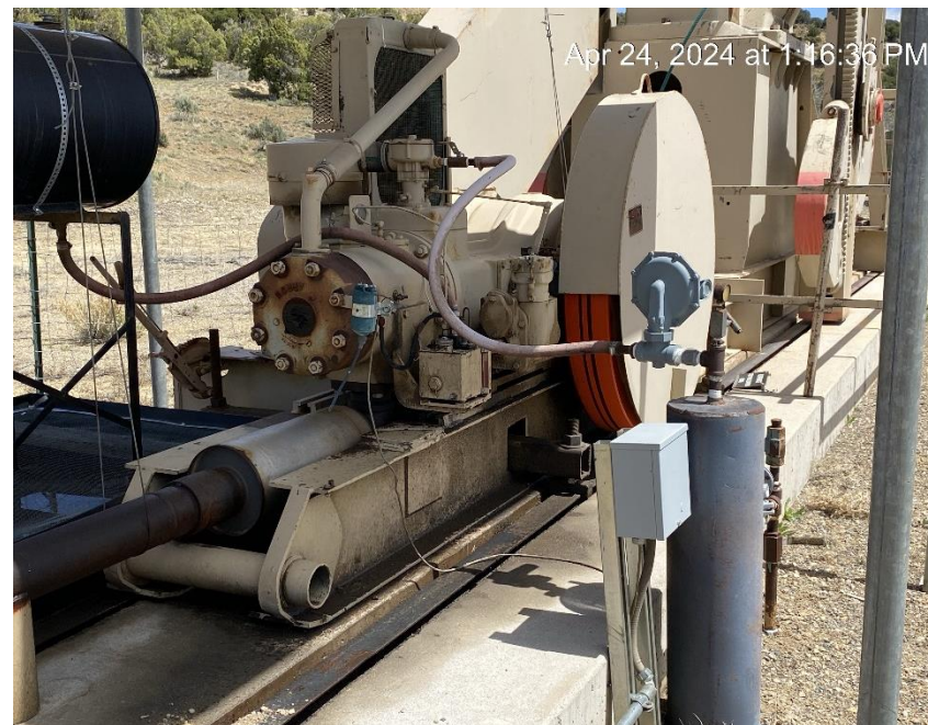
Oil leaks on engine
