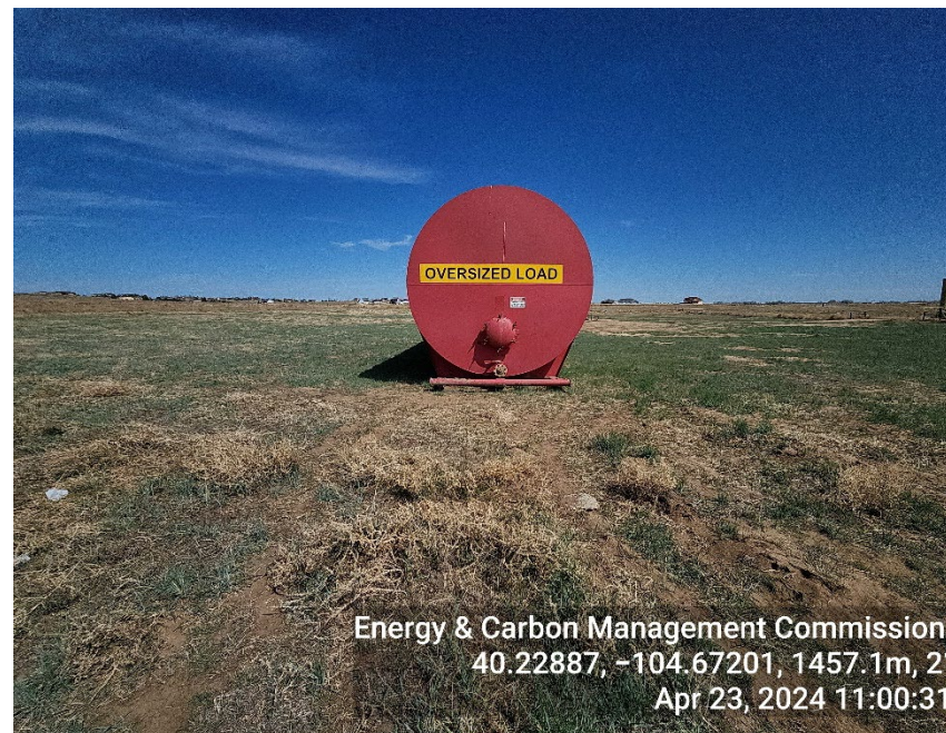
Photo 4: no grounding rod/berm
