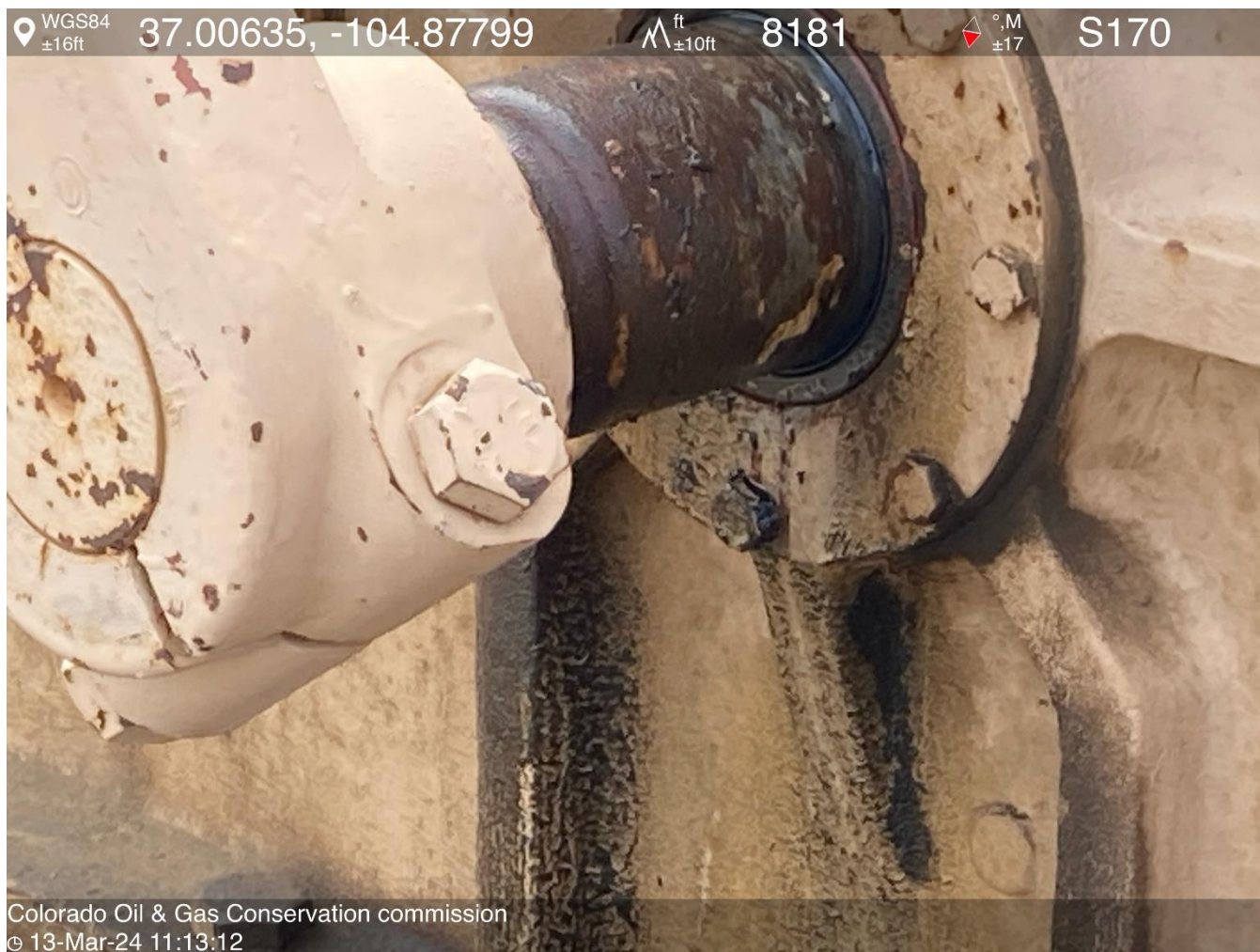
PHOTO 7: LEAK ON PUMPJACK GEAR BOX APPEARS TO BE THE SOURCE OF OILY WASTE IMPACTING SOILS AROUND PUMPMACK. Securely fasten all valves, pipes, fittings, and Production Facilities to ensure good mechanical condition, inspect at regular intervals and maintain in good mechanical condition per Rule 608.e. CA DATE 5-22-2024.
