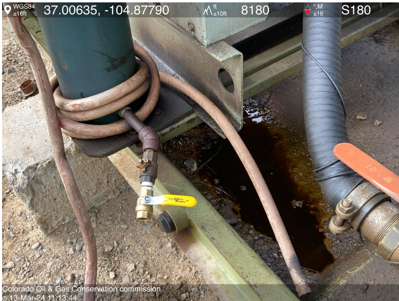
PHOTO 8: OILY WASTE INSIDE PRIME MOVER SECONDARY CONTAINMENT (ENGINE SKID). COMPLY WITH RULE 1002.f.(2)B, Comply with general provisions of the oil and gas act for wildlife protection AND SB-181. CA DATE 4-23-2024.
