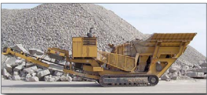
Figure 6. Crushed concrete stockpile and crusher
