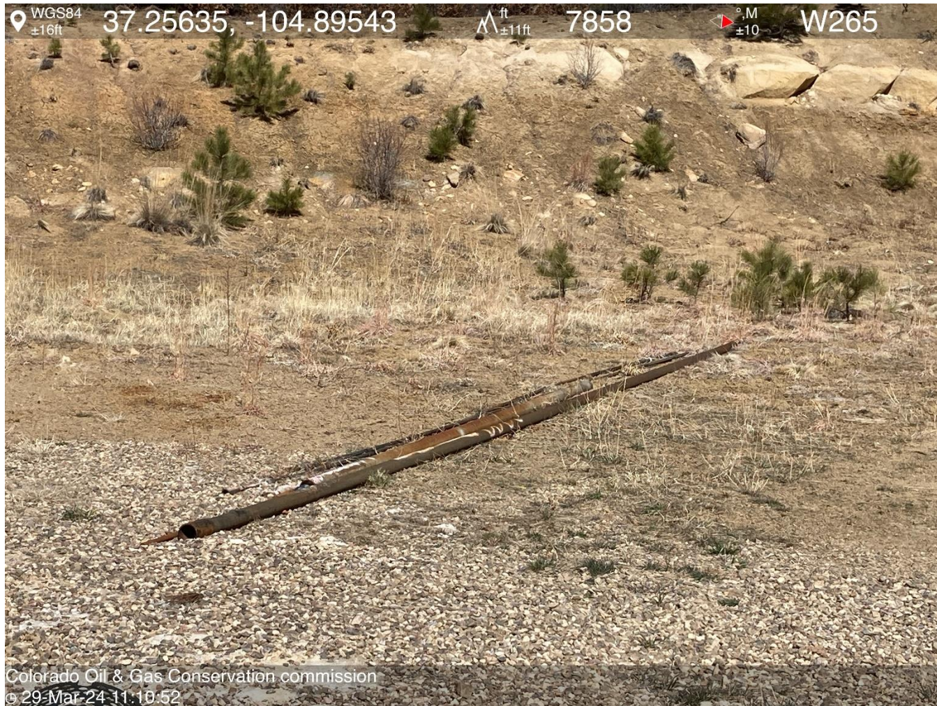
PHOTO 4: UNUSED EQUIPMENT STORED ON LOCATION (TBG & RODS). REMOVE UNUSED EQUIPMENT PER RULE 606. CA DATE 5-20-2024.
