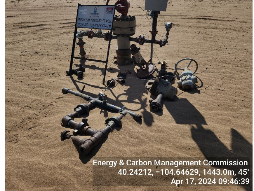
Photo 4: Unused/disconnected equipment
