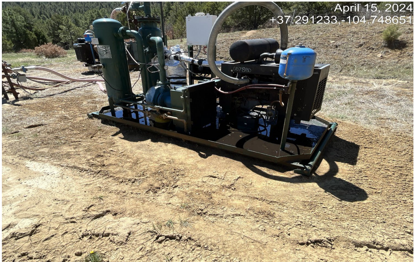
Photo 4. There is oil in the engine skid that needs to be cleaned up..
