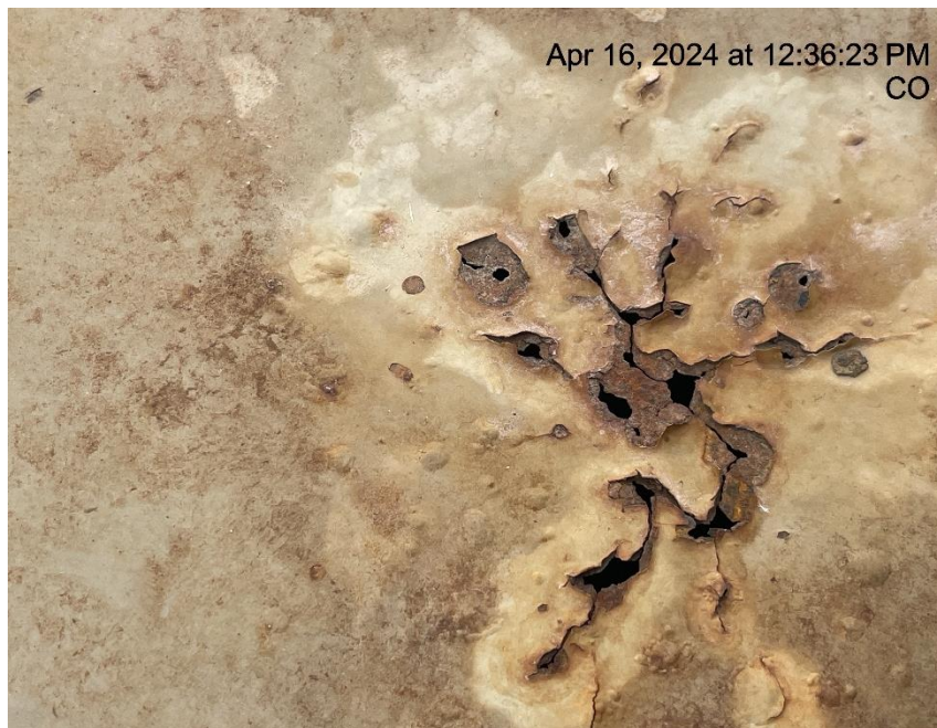
Photo # 4189 Possible tank failure – tank appears to be compromised, holes & corrosion on the top of tank
