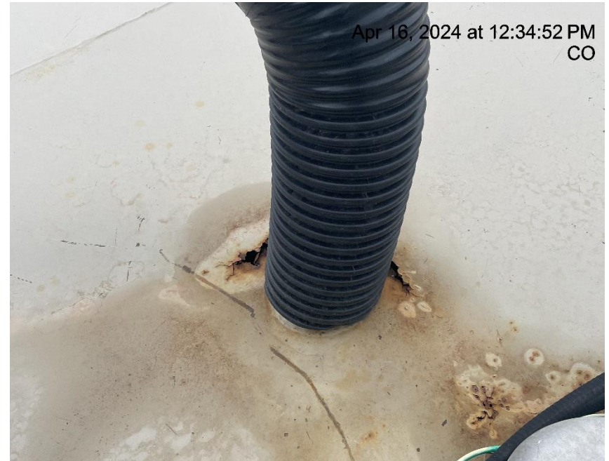
Photo # 4192 Possible tank failure – tank appears to be compromised, holes & corrosion on the top of tank
